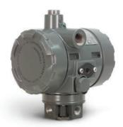
Electro-Pneumatic (I/P) Transducers convert an electronic signal to a pneumatic signal. They are routinely used in control loops that require an electronic control signal from a programmable logic controller or distributed control system to be converted to a usable pneumatic signal for operation of a control valve. I/P transducers operate by using a current to pneumatic converter to produce a proportional pneumatic output.
