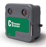
Pneumatic Controllers are mechanical devices designed to measure temperature or pressure and transmit a corrective air signal to the final control element. Bourdon tubes, bellows, temperature elements, or displacers are used as the sensing elements. The power supply and output of a pneumatic controller is compressed air or natural gas.
