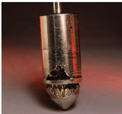
Figure 5.8 Typical Appearance of Flashing Damage
