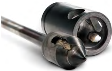
Figure 5.9 Typical Appearance of Cavitation Damage
